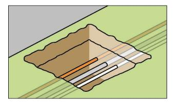
Figure 1: Underground essential services exposed by 'potholing'.
